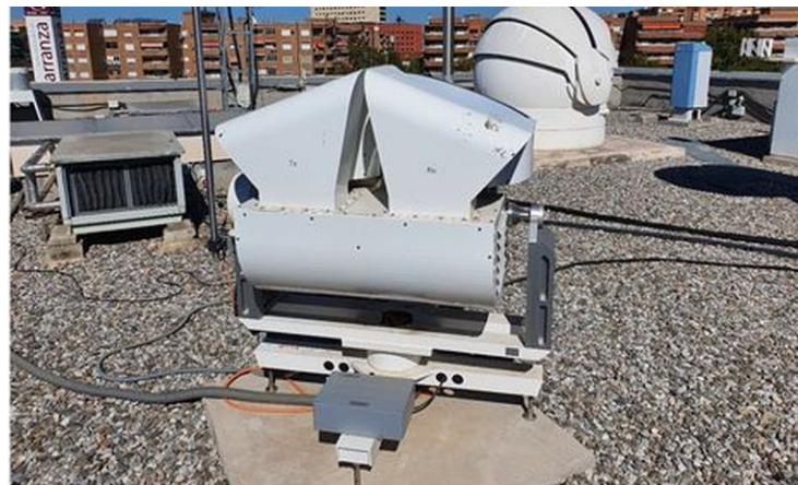
Radar Doppler de nubes (RPG-FMCW-94-DP)
